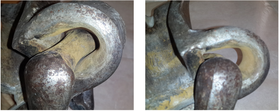
Figure 6. Wear of connecting link and track lug
