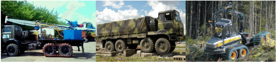
Figure 1. Vehicles, which may be equipped with bogie tracks. a – transport, b – military, c – timber harvesting
