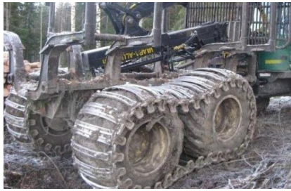
Figure 7. Standard bogie track sagging
